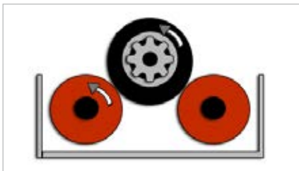
Easy-drive-out-system: To leave the roller set faster, only in conjunction with rotation and measurement direction reversal
