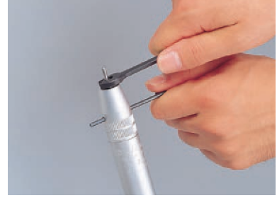
Fasten the collet chuck firmly to avoid loosening of the cutting tool.
